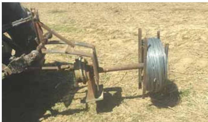
Pto-operated wire winder mounts on a home-built steel frame. An old car wheel rim contains the wire.
