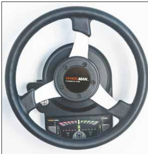
Autosteer bracket slides into place around tractor's steering column and contains a small electric motor to steer tractor. A dashboard with light bar attaches to bracket.
