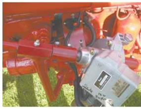
Electric steering unit is mounted to a custom-made base plate that's bolted to tractor's bell housing.
