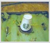
Gary Swensen, Yankton, S. Dak.: "When I use my gooseneck trailer, I like to put some grease on the ball. When it's not in use the grease collects dirt and leaves. This little coffee cup solves the problem.3
