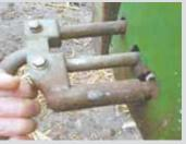
were out, it would snap back in again. So I would have to get off the tractor and pull it out again. I solved the problem by building up the rounded edge of the pin with weld and then grinding it smooth. The keyhole that the wider part of the pin turns into was punched in, making it slightly worn so I built that up as well. Now it takes a heck of a bump to
