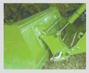
Fritz Groszkruger, Dumont, Iowa: "I've got a 'global attachment' quick-tach Deere front-end loader. To release attachments, you pull out the handle and turn. The problem I had was that if I hit a bump while the pins
