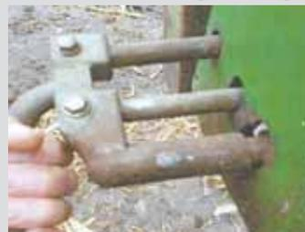
were out, it would snap back in again. So I would have to get off the tractor and pull it out again. I solved the problem by building up the rounded edge of the pin with weld and then grinding it smooth. The keyhole that the wider part of the pin turns into was punched in, making it slightly worn so I built that up as well. Now it takes a heck of a bump to pop it back in.”
