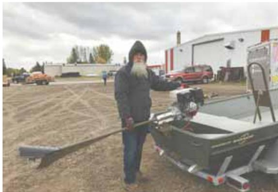
SWOMP shallow water motor will propel boat through the shallowest waters and thick debris without plugging up.
