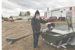
SWOMP shallow water motor will propel boat through the shallowest waters and thick debris without plugging up.
