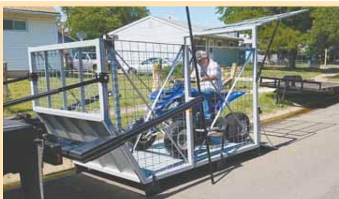
**Self-contained livestock pen is loaded and unloaded by the bale handling arms on Reinert's pickup-mounted Hydra-Bed bale hauler.**
