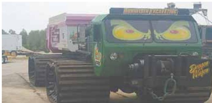
**Built-from-scratch, articulated dump truck measures 37 ft. long and rides on 4 sets of rubber tracks. The cab is off an old Army tank retriever.**
