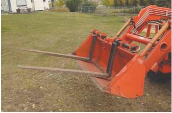
Bucket forklift was made by welding 3 round brackets with holes in them on top edge of bucket, and welding brackets on top of 2 L-shaped forks. Steel rods run th brackets to support forks.
