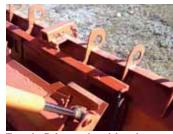
To make Bobcat-style quick-tach system, McNaughton welded a quick-tach receiver plate on back of bucket and matching pick up" brackets on loader.
