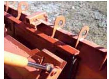
To make Bobcat-style quick-tach system, McNaughton welded a quick-tach receiver plate on back of bucket and matching "pick up" brackets on loader.
