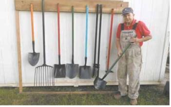
"I use the top rails off chain link fences to make handles for garden tools. They're stronger and don't break as easily as wood," says Dan Long.
