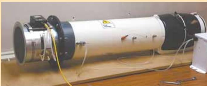
Plasma purifier produces electric discharges that sterilize incoming air, protecting pigs from viral and bacterial-based diseases.
