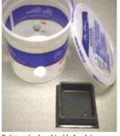
Bait tray is placed inside 1-gal. ice cream container with 4 evenly spaced holes cut into it.
