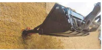
Hydraulic-operated rotating teeth on bucket fold out to tear silage off face of bunker silo.
