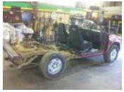
Martin cut off Blazer's body behind the bucket seats, keeping the frame and running gear.
