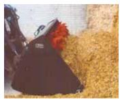
By folding teeth back in, operator can load bucket with loose silage.
