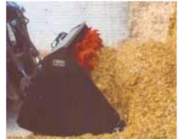
By folding teeth back in, operator can load bucket with loose silage.
