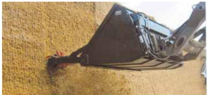
Hydraulic-operated rotating teeth on bucket fold out to tear silage off face of bunker silo.
