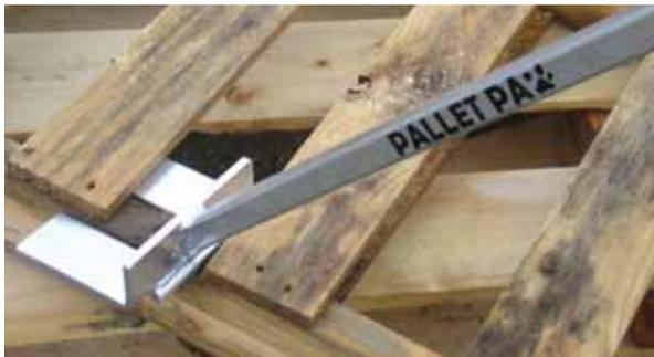
Pallet Paw uses 4-in. long steel "paws" welded on at an angle to tear pallets apart.
