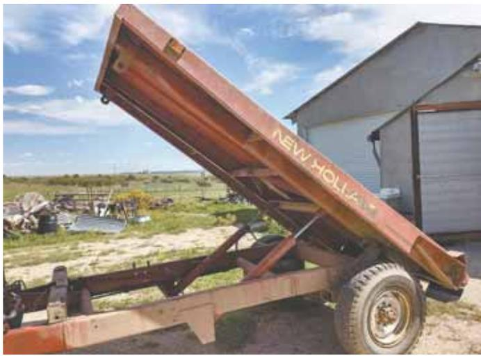
Eddie Angelovich used the back part of the bed on an old New Holland pull-type, small square bale wagon to build this hydraulic-operated dump trailer.
