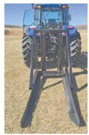
Steel pegs on rotating drums up front flake hay off between tractor and bale.
