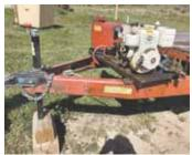
Hydraulic pump mounted on trailer tongue operates cylinders that raise and lower bed.
