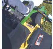
Marker system makes use of a can of water-based marking paint. System is turned on or off by a foot-operated switch.
