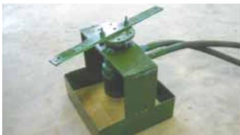
"Lump Buster" uses an 18-in. long steel blade to break up chunks of grain before they reach bin's auger.
