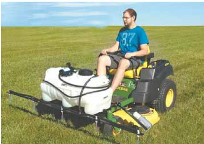
Front-mount sprayer for zero-turn mowers comes with a 100-in. boom and a spray wand. A foot-operated switch is used to turn sprayer on or off.
