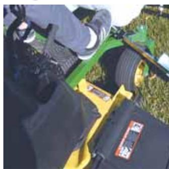
Marker system makes use of a can of water-based marking paint. System is turned on or off by a foot-operated switch.
