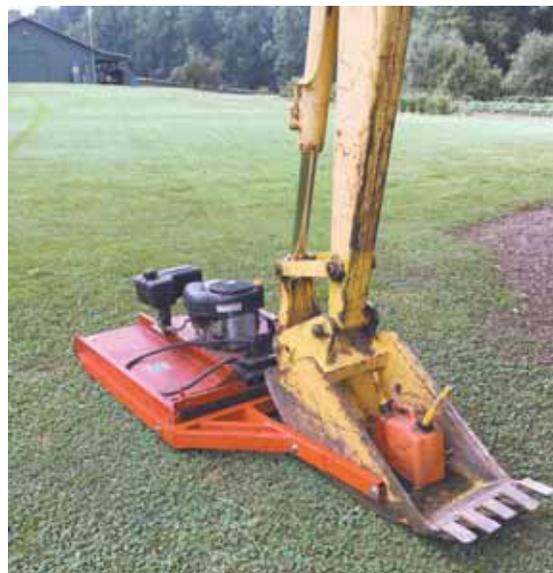
Backhoe-mounted mower can reach out up to 25 ft., allowing Lyle to safely mow grass and weeds in hard-to-reach areas around ponds and creek banks.
