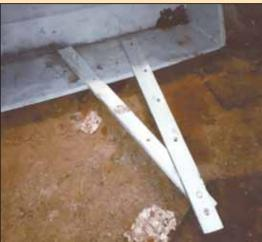
Worn-out grader blades measure 5 ft. long by 5 in. wide. Foellmi can either bolt them together in front or set them parallel like forks.
