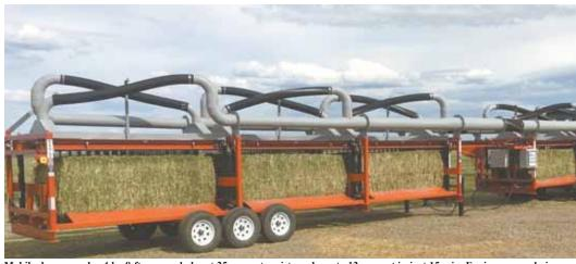
Mobile dryer can dry 4 by 8-ft. square bales at 25 percent moisture down to 12 percent in just 15 min. Engine-warmed air, compressed by a fan, is driven into the hay.
