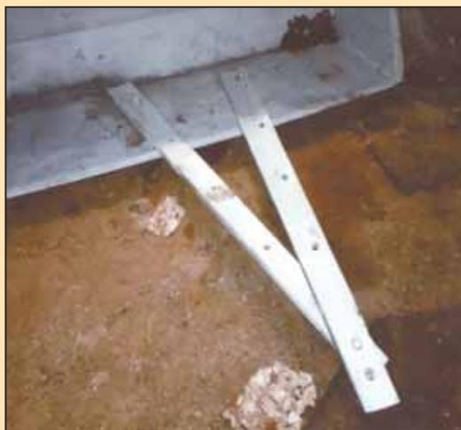
Worn-out grader blades measure 5 ft. long by 5 in. wide. Foellmi can either bolt them together in front or set them parallel like forks.
