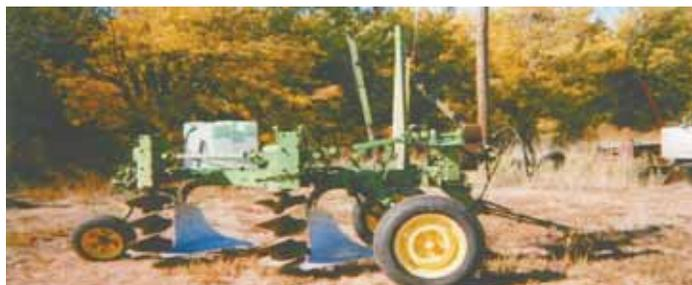
John Moellering is still using the whirlwind terrace plow he built 36 years ago. Slices of sod feed into vertical augers that throw the dirt up to 30 ft.
