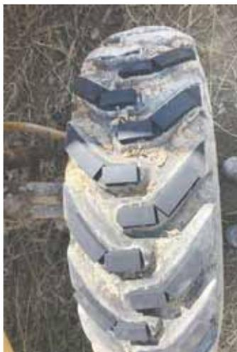
Pieces of pre-cut rubber tread glue on right over tire’s existing treads to boost traction.
