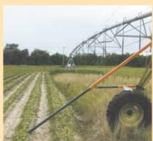
Pivot Pro works like a telescoping bicycle "kickstand" to brace against high winds.
