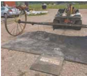
Conveyor belting hangs by chains from wheel rake axle.
