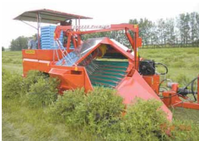
**Pull-type combine harvests half a row of haskap or aronia berries with each pass. Tines shake berries loose from bushes to drop onto a conveyor, which carries them to boxes on a rear platform.**
