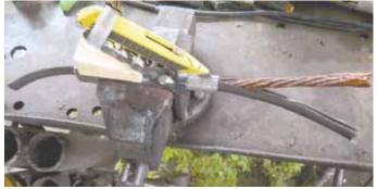
Sid Stubbs uses his bench vise-mounted cable stripper to remove the rubber from battery cables. "I can strip a lot of cables in a very short time," he says.
