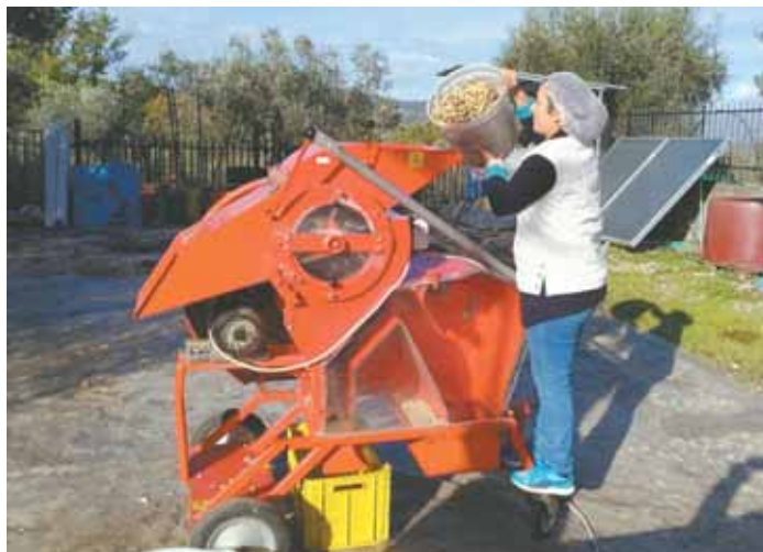
Imported by Eugene Canales, this Cicoria stationary small plot thresher comes with 6 different sieves. Works great for grains, as well as legumes and even vegetables.
