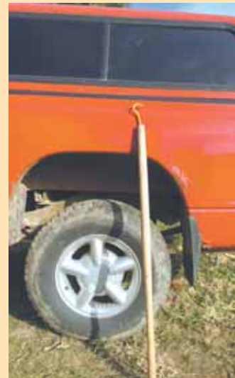
Ruen drilled a hole in the end of an old spade handle and screwed a plastic-covered hook into it.
