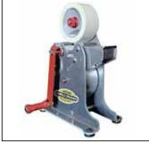
Canola crusher presses crushed seed in neat rows onto masking tape that feeds out back of device.
