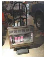
Wall-mount, non-vent propane residential heater straps onto 2-wheeler where it can be easily moved anywhere in Payne's shop.
