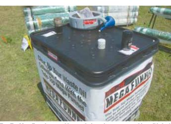
Tote-Top Mega Funnel comes with a punched metal screen on top with a solid plastic layer beneath it that funnels drain oil down into tote for later disposal.
