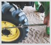
Dave Meiners, Edgerton, Minn.: "I had a hard time using a box end-open end wrench in order to break the stud bolts loose on my tractor's front wheels. To gain more leverage, I hooked the box end of a second, slightly larger wrench into the open end of the first wrench. As soon as I applied pressure, the bolts immediately popped loose."
