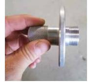
Oil filter removal tool threads onto filter. A 3-in. dia. disc on top seals against filter O-ring.
