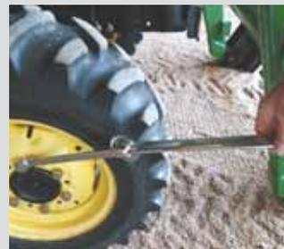
**Dave Meiners, Edgerton, Minn.:** "I had a hard time using a box end-open end wrench in order to break the stud bolts loose on my tractor's front wheels. To gain more leverage, I hooked the box end of a second, slightly larger wrench into the open end of the first wrench. As soon as I applied pressure, the bolts immediately popped loose."
