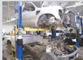
Ford dealership. He let me come in one day to take pictures of the mechanics working on a truck engine. It's a lot different working on a truck engine today than it was back in the old days when we put a hoist up in a tree to pull the engine. Now they lift the entire body off the chassis. All the wiring has quick disconnects. About a dozen bolts connect the cab to the frame.
