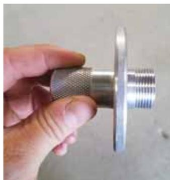
**Oil filter removal tool threads onto filter. A 3-in. dia. disc on top seals against filter O-ring.**
