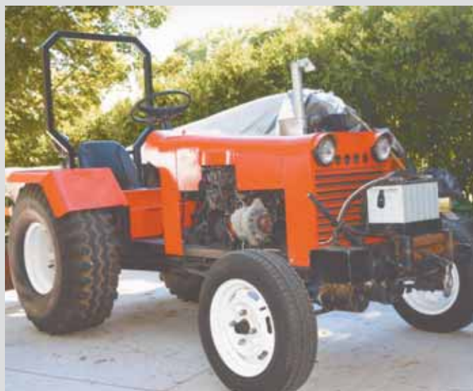
An electric winch on the front end is used to pull logs and also "unstuck" the tractor, if needed. A battery next to the winch gives it plenty of power.
