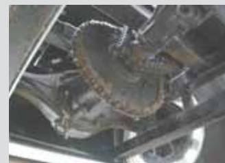
To slow down the tractor's drive speed, he mounted a jackshaft with large and small sprockets alongside the driveshaft.
