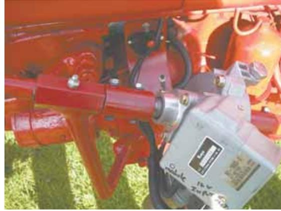
Electric steering unit is mounted to a custom-made base plate that's bolted to tractor's bell housing.
