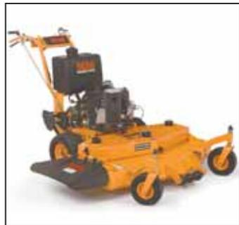
**Gary Eichhorn, Parkersburg, W. Va.:** Gary's impressed with his 2012 **Scag** walk-behind mower equipped with a 16 hp. Briggs & Stratton engine and 48-in. deck. "My neighbor and I start mowing our 2-plus acre fields at the same time. I walk, and he uses a riding mower. He goes faster up and down the field, but I get done a half hour sooner because of the big deck."
