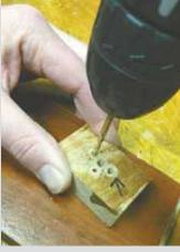
Ryan Van Der Bill, Sioux Falls, S. Dak.: "One idea is that when you need to drill a straight hole and you don't trust your eye with a hand drill, take a small block of oak or maple and drill a hole through it with a drill press. Then use that block as a guide when using a hand drill."
