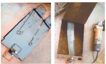
Fisher cut into the deck on his bush hog mower and installed an 8 by 12-in. hinged access door. "I remove a bolt and flip the door up, then use a grinder to sharpen the blades," he says.
