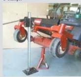
Andy Kozlowski, Califon, N.J.: "I use a car bumper jack from the 1970's to lift my zero-turn mower so I can clean the deck and sharpen blades. I put a ring on the bumper jack's hook and then put an
