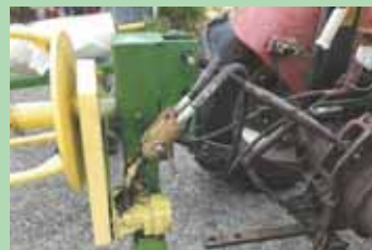
Cornett used a commercial hydraulic-driven bale spear to make his wrapper.
