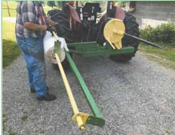
Cornett moves roll of plastic back and forth as bale spins on spear.
