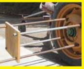
Last winter FARM SHOW published a story on how I used one of the rear wheels on my tractor to make a wheelmounted winder for old fence wire (Vol. 42, No. 2). I screwed four 10-in. long pipes to studs on the wheels and then jacked up the wheel and put the tractor in gear. It works great and results in neat, reusable wire rolls.
