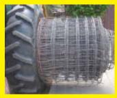
concept. I inserted 3-ft. lengths of 1-in. dia. pipe into each of the four original pipes, then slid on a plywood board with holes drilled into it to match the pipes. Within 10 min. I had all 300 ft. of fence neatly rolled. Then I just knocked the board off the pipes and slipped the wire roll off. (Don Buelke, 2351 Vista Ridge, Victor, Mont. 59875 ph 406 381-4766; donbuelke@gmail.com)
