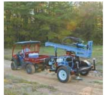
Lone Star offers both mechanical and hydraulic drills for wells up to 400 ft. deep. Options include down hole hammers, and roller cone bits for rocky areas.
