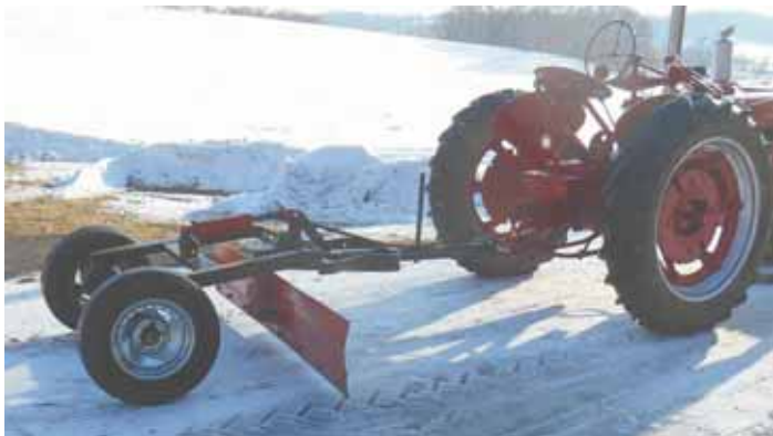
"It does a better job of leveling because it rides on wheels and because the frame is twice as long as before," says Tim Mounce.
