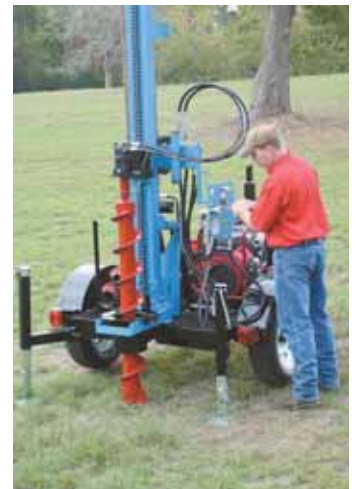
Lone Star offers both mechanical and hydraulic drills for wells up to 400 ft. deep. Options include down hole hammers, and roller cone bits for rocky areas.
