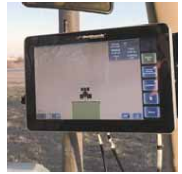
Rebel autosteer system can be used on tractors dating back to the late 1970's.
