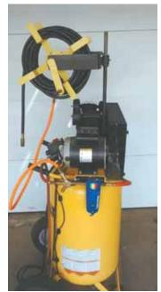
Swivel allows compressor-mounted hose reel to rotate freely in any direction.
