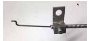
To repair the outer sleeve of a broken control cable you can use a variety of electrical connectors to secure one cable sleeve to another, says Roger Podoll. They include an inline union (above left) and a single set screw inline lug (above). Another quick fix uses ground wire clamps.
