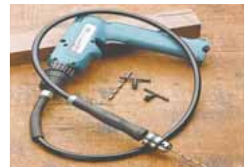
Bosch drill bit sharpener consists of a grinding wheel powered by a drill (left). Faithfull's flexible driveshaft extends the reach of a power drill.
