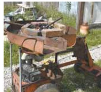
Blackford flipped mower deck upside down, then welded it to a stand to serve as the firebox for his mobile forge.
