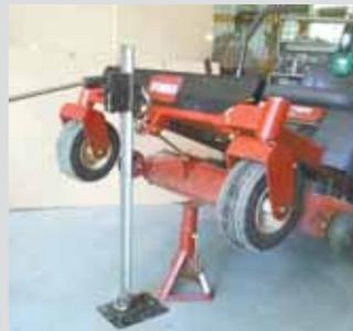
**Andy Kozlowski, Califon, N.J.:** “I use a car bumper jack from the 1970’s to lift my zero-turn mower so I can clean the deck and sharpen blades. I put a ring on the bumper jack’s hook and then put an S-hook on that. I place a jack stand under the deck for safety. Best of all, the bumper jack takes up little space when not being used.”
