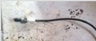
**Russell Nemsch, Thorndale, Texas:** “Here’s an idea I use when I need to change spark plugs but don’t have much room to maneuver. I attach a piece of 3/16-in. dia. vacuum hose onto the plug and then thread it into place. Twisting the spark plug this way gives me a good sense of feel so I don’t accidentally strip the threads.”
