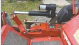
**John Travis, Dundee, N.Y.:** “The pedal that’s used to raise or lower the 60-in. deck on my Ferris zero-turn riding mower was hard to push down, so hard that I eventually suffered a torn meniscus knee injury. Ferris makes a deck lift assist for some of their mowers but not mine. My neighbor, who owns a fabrication shop, suggested we could use an electro-hydraulic cylinder from an old Deere small square bale thrower to raise or lower the deck automatically.
