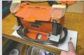
“Here’s another shop idea. If you have a small bench grinder or other tool that you don’t want to mount permanently on your workbench, mount it to a piece of plywood fitted with a couple screws that you can use to hold it tightly on your workbench when needed. Quicker and easier than using C-clamps.”
