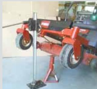
**Andy Kozlowski, Califon, N.J.:** “I use a car bumper jack from the 1970’s to lift my zero-turn mower so I can clean the deck and sharpen blades. I put a ring on the bumper jack’s hook and then put an S-hook on that. I place a jack stand under the deck for safety. Best of all, the bumper jack takes up little space when not being used.”
