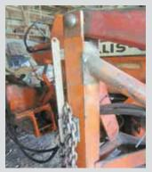
Andy Nelson, Webster, Minn.: "I wanted a handy place to store chains on my Allis Chalmers 170 loader tractor, so I bolted an angle iron bracket onto one of the loader arm uprights and then bolted an 18in. long, 2-in, wide metal strap vertically onto it. I just drop chains into a small gap between the strap and upright so they hang down from the angle iron. Works great.
