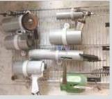
**Donald Chapman, Billings, Mo.:** "I mounted a 4-ft. long by 20-in. wire rack on my shop wall to make a handy air tool storage rack. I cut up lengths of pvc electric conduit in order to make customized tool holders that are supported by pvc conduit hangers. I also cut notches into each holder to make room for the tool's handle.
