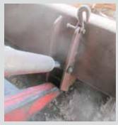
"I also bolted a pair of chain hooks on back of the loader bucket, which I use with a chain to drag logs out of the woods. I drilled holes in the mounting brackets that support the bucket cylinder, then slipped each hook over the top of the bracket and inserted a bolt."
