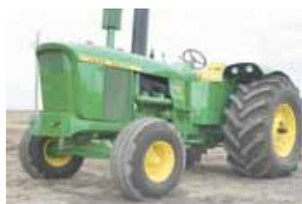
**Spindles on this Deere 4020 loader tractor were replaced with the heavier front end from a Deere 5010.**
