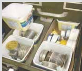
"One idea is to use the cardboard cartons that hold new spools of MIG welding wire. The boxes are about 14 in. square, and by splitting them in half and flipping them upside down, you have 2 instant bins that will fit neatly into cabinet drawers. Plastic margarine containers or baby wipe containers can be placed inside them."
