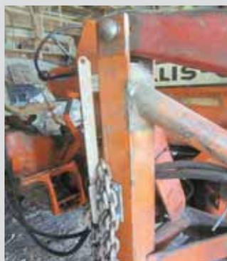
**Andy Nelson, Webster, Minn.:** "I wanted a handy place to store chains on my Allis Chalmers 170 loader tractor, so I bolted an angle iron bracket onto one of the loader arm uprights and then bolted an 18-in. long, 2-in. wide metal strap vertically onto it. I just drop chains into a small gap between the strap and upright so they hang down from the angle iron. Works great."
