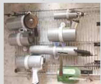
**Donald Chapman, Billings, Mo.:** "I mounted a 4-ft. long by 20-in. wire rack on my shop wall to make a handy air tool storage rack. I cut up lengths of pvc electric conduit in order to make customized tool holders that are supported by pvc conduit hangers. I also cut notches into each holder to make room for the tool's handle."
