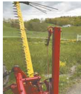
Cornett welded a 3-in. chain link on back of sicklebar. A hook on winch cable attaches to link to raise and lower sicklebar.
