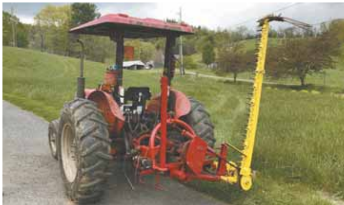
Cornett welded a winch onto a steel plate that he bolted to left side of mower. He welded a 5-ft. length of square tubing to the same plate, fitted with a 3-in. pulley.
