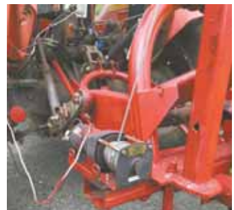
Cornett welded a 3-in. chain link on back of sicklebar. A hook on winch cable attaches to link to raise and lower sicklebar.
