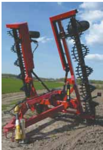
Folding Stone Windrower sweeps up to 12-in. dia. rocks into a 5-ft. wide windrow. At 28 ft. wide, it covers a lot of ground fast.
