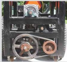
Jeff Kohl wanted a ptodriven generator on hand in case the electric power went out, but didn't want his tractor's engine to run at full throttle for a long time. So he built a 3-pt. mounted unit and fitted it with a 540 rpm pto shaft and a series of V-belts.
