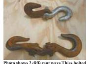
a chain hook and grab hook together to lift heavy loads with his chain hoist
