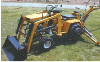
Adding hydraulics to a garden tractor can multiply its engine power by 1,000 times or more, allowing you to do many jobs not possible before, says Norman Ng.
