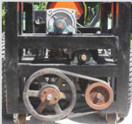
Jeff Kohl wanted a pto-driven generator on hand in case the electric power went out, but didn't want his tractor's engine to run at full throttle for a long time. So he built a 3-pt. mounted unit and fitted it with a 540 rpm pto shaft and a series of V-belts.
