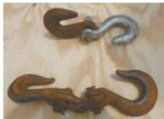
Photo shows 2 different ways Thies bolted a chain hook and grab hook together to lift heavy loads with his chain hoist.
