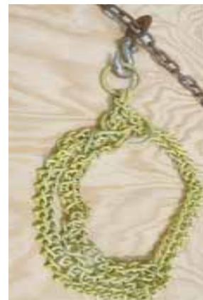
Grab hook keeps load from shifting on chain. Thies uses the hooks for a variety of jobs around the farm.
