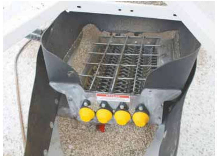
LumpBuster auger attachment fits inside the auger hopper under a fertilizer bin, breaking up lumps before you load up to head to the field.
