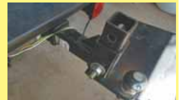
Swensen welded a short length of vertical tubing to his truck’s existing receiver hitch.
