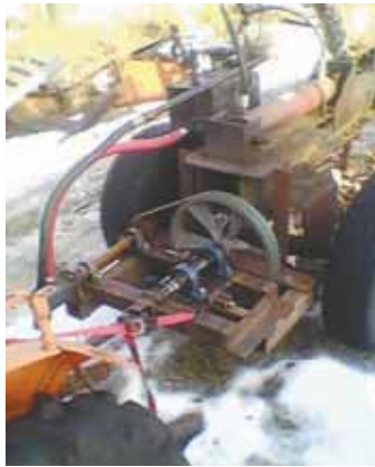
Larry St. Germain converted his wood splitter to pto drive using the stub shaft from a pto-driven gearbox and the pulley off an old air compressor.
