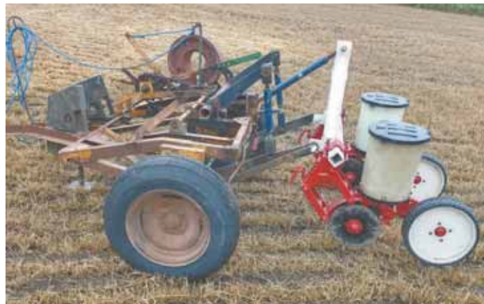
Jacob stripped grain drill down to make a tow-behind caddy, then added a 3-pt. hitch that attaches to drill's mechanical lift. He pulls a trip rope to raise or lower planter.
