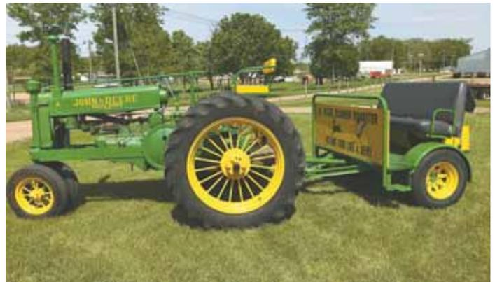
Pto-powered cart is built on a Roadster axle. When Wilson wants to travel faster than his tractor can, he puts the pto in gear and takes the tractor transmission out of gear.
