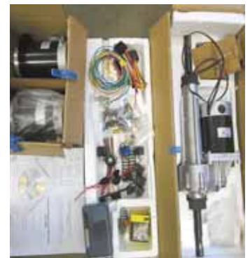
Other kit components include an electronic motor controller, control relays, digital amp/volt meter, circuit breakers and more.
