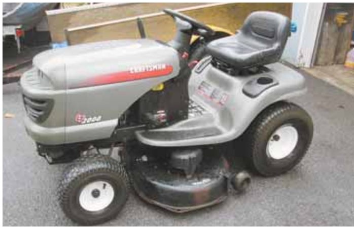
Brian Edmond put together a complete kit for converting a 38 to 42-in., gas-powered lawn tractor to 24-volt all-electric drive.
