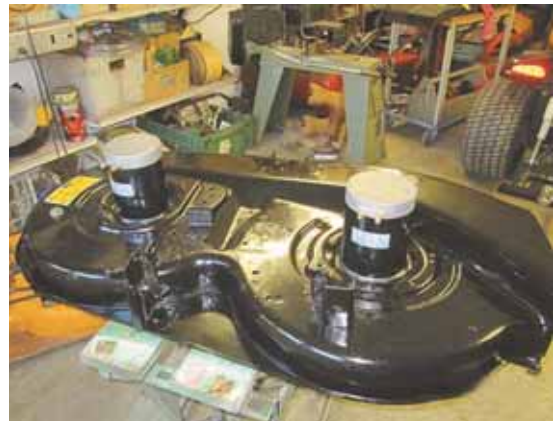
Kit includes individual motors with mounting flanges for blade drives. Power to the motors on each blade is delivered via a plug-in cable.
